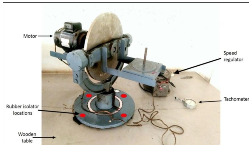
Fig. 1 Gyroscope coupled with varying speed motor experimental setup
